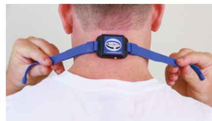
Figure 3. A vibratory sleep device placed around the neck which vibrates when patient is in supine position. Vibration will stop when patient rolls out of supine position. Image courtesy of Nightshift.
